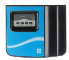
The **Testomat**<sup>®</sup> **808** is a compact analyzer for online measurement of water hardness according to the principle of "limit value monitoring with color change" in the measuring range 0.02 - 5 ° dH (0.4 - 89 ppm).
