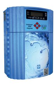
The **Testomat 2000® Polymer** process photometer is an online analytical instrument for monitoring the content of polyacrylate in the range from 0 to 50 mg/l (ppm) (with a set product-specific factor of 1.00) using the photometric analysis principle.
