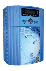
The **Testomat 2000**® **Fe** process photometer is an online analytical instrument for monitoring the dissolved iron (II) + (III) content in the range from 0 to 1.0 mg/l (ppm) using the photometric analysis principle.
