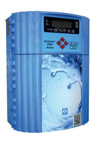
The **Testomat 2000® Antox** is a special version of the Testomat 2000® with an additional pump for dosing a reducing agent. By adding this reducing agent to the already filled measuring chamber, the interference caused by oxidizing agents is eliminated. Further analysis of the water hardness measurement is then continued according to the standard procedure.
