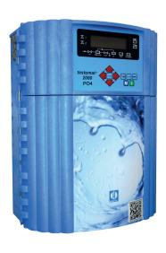
The **Testomat 2000**® **PO**<sub>4</sub> process photometer is an online analytical measuring instrument for monitoring the content of ortho-phosphate in the range from 0 to 10.0 mg/l (ppm) using the photometric analysis principle.
