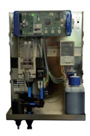
The **Testomat® LAB TH** determines the water hardness fully automatically by means of titration. The device is suitable for checking the water quality of water treatment plants, drinking water plants, industrial boilers and for monitoring process water.
