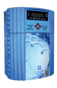
The **Testomat 2000**® **CLT Self Clean** process photometer with additional cleaning function for the measuring chamber is an online analyzer for monitoring the content of total chlorine (CLT) in the range of 0-2.5 mg/l (ppm); switchable to free chlorine in the same measuring range.
