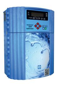
The **Testomat 2000 THCI**® bprocess photometer determines the content of total chlorine according to the photometric analysis principle in the range from 0 to 2.5 mg/l (ppm) and the water hardness in the range from 0.25 to 2.5° dH by titration.
