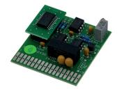
Current interface SK910 for Testomat 2000® / Titromat® Power interface (plug-in card)
